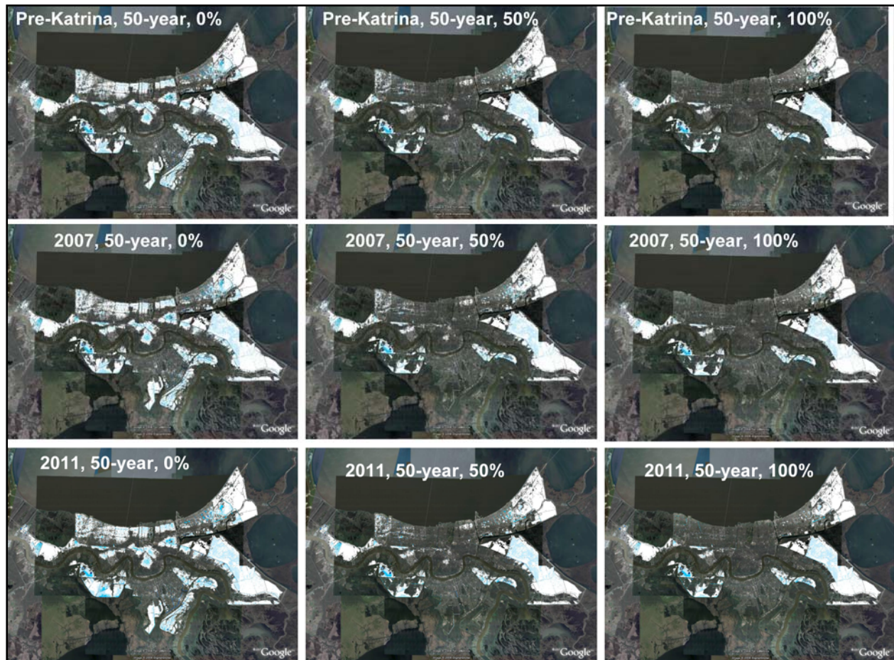
Figure 15. Flood Depth Frequency Maps for 50-Year (2%) Hurricane Floodplain, showing impact of different pumping capacities. The label on each map indicates the HSDRRS infrastructure, flood frequency and percent pumping capacity modeled.
